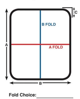
An "A Fold" cuts the A dimension in half, a "B Fold" cuts the B dimension in half.
